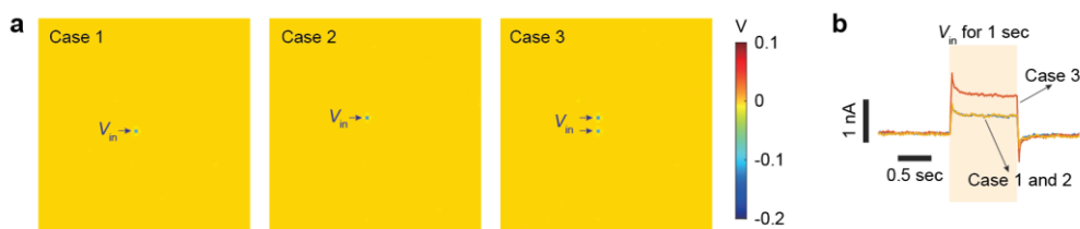
Figure S6. Another additional interference testing. (a) For Case 1 and 2, we apply a V_{in} pulse (amplitude = -0.08 V) to only pixel 9 and only pixel 8 (which belong to the same column), respectively. For Case 3, we apply the same V_{in} pulse (amplitude = -0.08 V) to both pixel 9 and pixel 8 simultaneously. I_g = 0 for all pixels for all three cases. (b) The measured I_{out} 's for Case 1 and Case 2 are nearly identical and the measured I_{out} for Case 3 is the same as the sum of I_{out} 's for Case 1 and Case 2. This shows that the two activated center disks with I_g = 0 do not interfere with each other.
